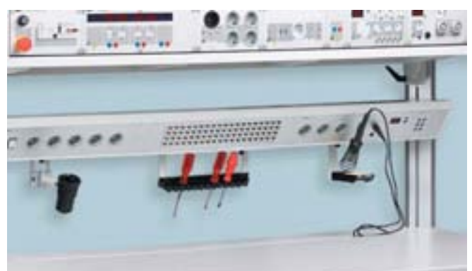
On the back of an adaptable aluminium profile further functions can be attached to the system channel such as accumulator, tool storage, perforated metal sheets, rotary table for small articles, device platform etc. Due to the shelf for the soldering iron the iron floats above the table top. The soldering station is installed in the system channel. This creates personal space on the working place and things are tidied up.
