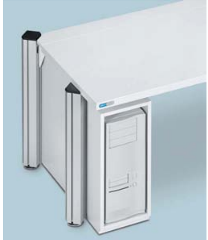
PC base cabinet, floor-mounted, of a system width of 270 mm, front height 680 mm. The PC base cabinet has a double wing door with integrated ventilation grate in the inside in the rear part. On request a lockable front door is deliverable.
